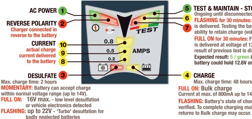
**TEST & MAINTAIN - STORAGE Ongoing until disconnected from battery** FLASHING for 30 minutes: NO charge is delivered. Testing the battery's ability to retain charge (voltage). FULL ON for 30 minutes: Float charge is delivered at voltage of 13.6V and result of previous test is displayed. Expected result: 5 / green indicates
